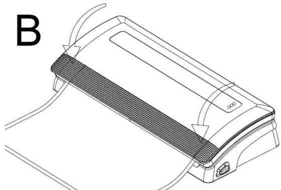
upper lid and press tightly on both sides of the cover by two hands (image B) till you hear motor working and, the device is now vacuuming to vacuum the bag (LED 9), and will seal the bag (LED 10), then stop when it is done fully automatically.
