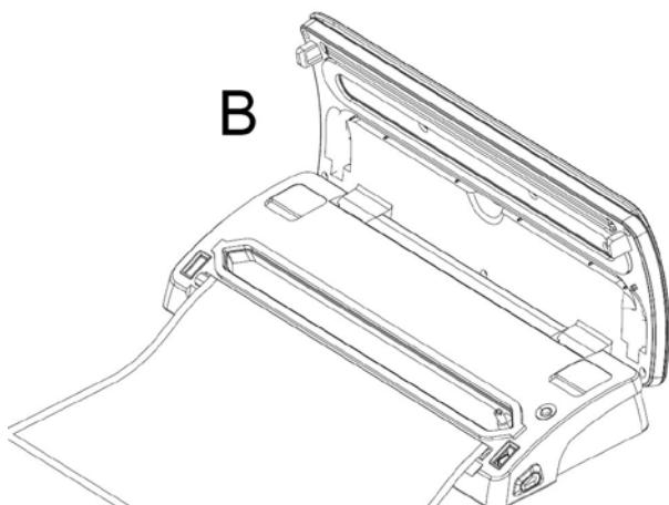
2. Put one end of the bag on top of the sealing profile (4) and the lower gasket (6) The open end of bag must not enter the vacuum chamber (5) (image B).
