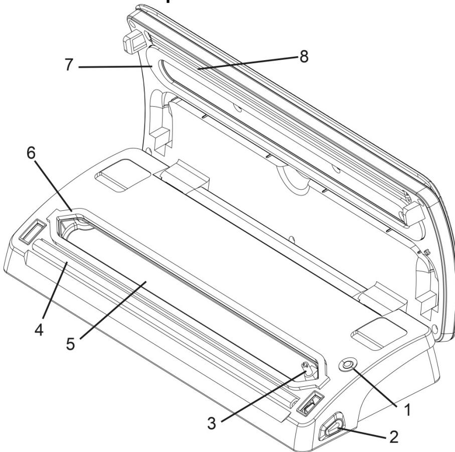
**1 Safety switch:** Is activated when the cover is closed.
